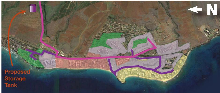
Fig. 5: Current capacity and proposed expansion of water reuse infrastructure in West Maui, and the properties served. At present, funding for design and construction of Option/Phase 1 and design for Option/Phase 2 properties has been secured; additional funding is necessary to further expand West Maui reuse capacity. Graphic adapted from County of Maui/Google Earth.
