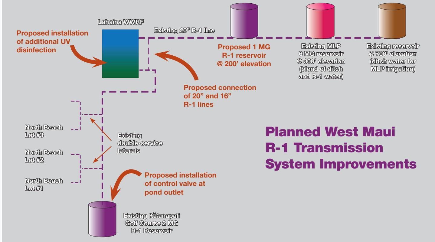
Fig. 6: Improvements to the LWRF currently underway to support the Option/Phase 1 infrastructure upgrades and expansion of reuse capacity. Image adapted from County of Maui.
