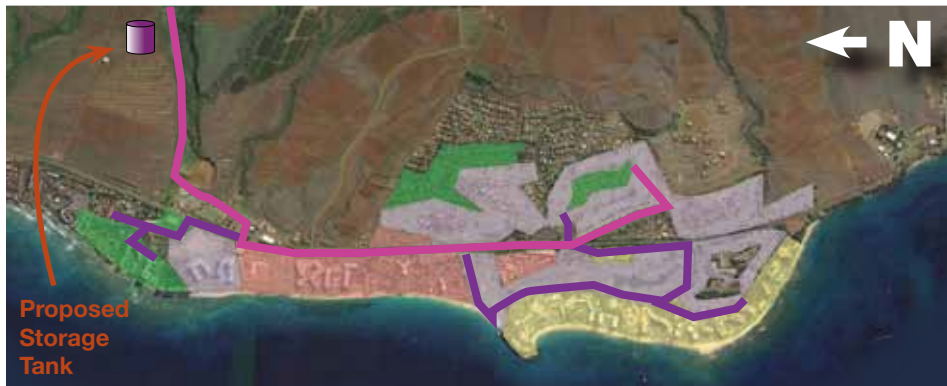
Fig. 5: Current capacity and proposed expansion of water reuse infrastructure in West Maui, and the properties served. At present, funding for design and construction of Option/Phase 1 and design for Option/Phase 2 properties has been secured; additional funding is necessary to further expand West Maui reuse capacity. Graphic adapted from County of Maui/Google Earth.
